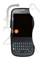
6 Run your thumbnail around the hairline opening to release the bottom-left and bottom clasps. End at (b).
