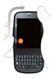
Run your thumbnail around the hairline opening to release the bottom-left and bottom clasps. End at (b).
