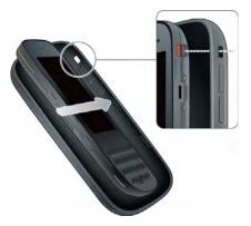
Press the back cover and the body of the phone together at each pair of clasps. You can feel the clasps engage.
