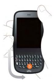
7 Swing the body of the phone out of the back cover as if the right side were a hinge.
