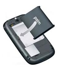
To replace the back cover: Insert the ringer switch into the hole provided for it on the right side of the back cover.
