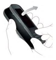
8 Remove the **battery** by sliding your finger under the groove at the side of the battery.
