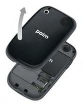
8 Remove the **battery** by pulling the tab that appears at the top of the battery.
