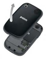
To remove the **battery**: Grasp the tab and pull it down and out to lift the battery out of the compartment.
