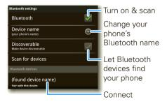
To connect with a new device, you need to pair with it. You only need to do this once for each device—to connect again, just turn on the device.
