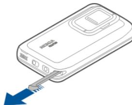
**Important:** Use only a stylus approved by Nokia for use with this device. Using any other stylus may invalidate any warranty applying to the device and may damage the touch screen. Avoid scratching the touch screen. Never use an actual pen or pencil or other sharp objects to write on the touch screen.
