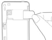
4. Please always remember to pull down the SIM card latch for locking your SIM card safely. If you don't pull down the SIM card latch, the device
