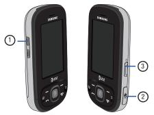
Volume keys: allows you to adjust the ringer volume while in standby mode or adjust the voice volume during a call. When receiving an incoming call, briefly press down either volume key ( ) to mute the ring tone. Press and hold either volume key to reject the call and send it directly to voicemail. Adjusts text size when reading a message or using the browser located in the Applications folder.
