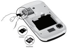
Note: The Samsung a687 has been tested to support up to a 16GB memory card.
