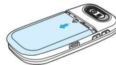
2. Insert the SIM card into the slot. The gold contacts of the SIM card should go against the metal contacts of the phone. Put the connector of the battery into the hole located at the top of the unit and then insert and press the lower side of the battery until you hear the light click. Make sure you align the gold contacts at the battery end with contacts on the phone. If the contacts at the battery are not properly aligned, damage could occur to the phone and the battery.
