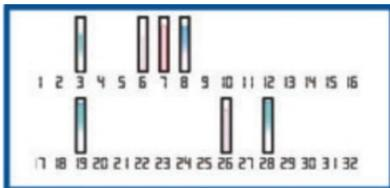
If your device has found satellites, a bar for each satellite is shown in the satellite information view. The longer the bar, the stronger the satellite signal. When your device has received enough data from the satellite signal to calculate your location, the colour of the bar changes.
