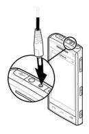
3 When the device indicates a full charge, disconnect the charger from the device, then from the wall outlet.
