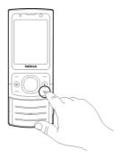
Press and hold the power key to switch the device on and off. Press the power key briefly to end a call or close an application.
