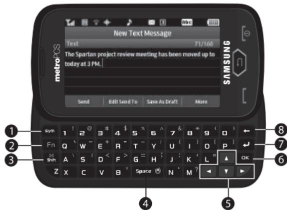
4. **Space / Vibrate Mode Key** — When entering text, press to insert a space. From the Home screen, press and hold to toggle between Normal Mode and Vibrate Mode.
