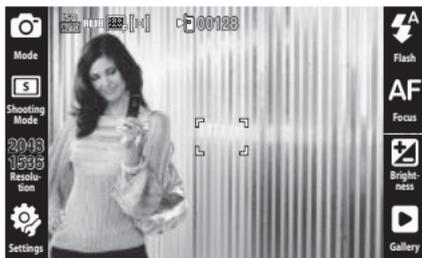
When you activate your phone's camera, the second line of the display is reserved for the current camera resolution setting and the picture counter. The center of the display shows a viewfinder image of the subject at which the camera is pointed.
