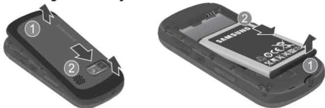
**Important!** You must unplug the adapter before removing the battery from the phone during charging to avoid damage.
