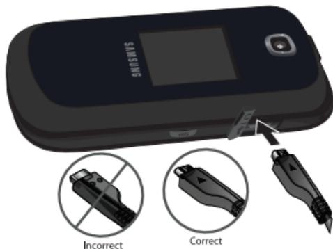
3. When charging is finished, remove the connector- from the interface connector jack on the phone.
