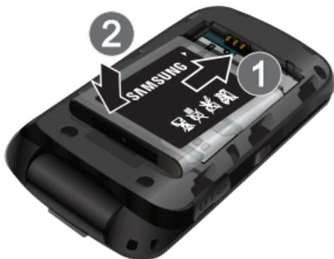
3. Replace the battery cover on the back of the phone (1) and slide it into place until you hear it securely click (2).
