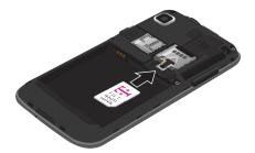
To remove the SIM card, carefully slide the SIM card out of the SIM card socket.
