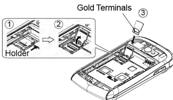
5. Replace the card and the card holder and gently press them, and then slide the holder in the direction of the arrow to lock it (4 to 6).
