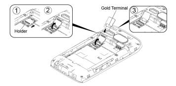
6. Replace the card holder and gently press it, and then slide the holder in the direction of arrow to lock it (4) and 5)
