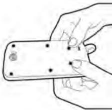
3. Finally, press two point on the left and right of back cover fully until hearing clicks.
