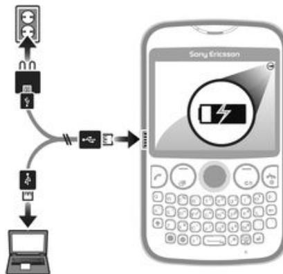
**To charge the phone using the power adapter**
