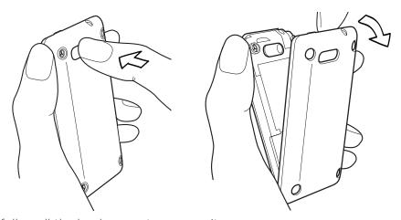
3. Carefully pull the back cover to remove it.
