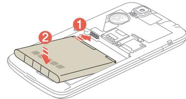
4. Slide the battery into the phone until it lays flat in the compartment.
