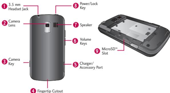
1. **3.5mm Headset Jack** allows you to plug in a headset for convenient, hands-free conversations. CAUTION! Inserting an accessory into the incorrect jack may damage the device.
