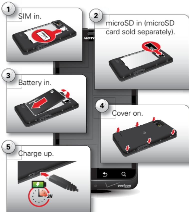
**Warning:** Please use only an approved charging accessory to charge your device. Improper handling of the charging port, as well as the use of an incompatible charger, may cause damage to your device and void your warranty.
