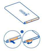
2 To unlock the SIM card holder, slide the holder to the left. Carefully pull out the holder.
