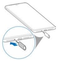
Pull out the card tray. You can place a nano-SIM card on the card slot 1, and place a nano-SIM card or a microSDXC card (optional) on the card slot 2, as shown. Carefully slide the tray back into place.
