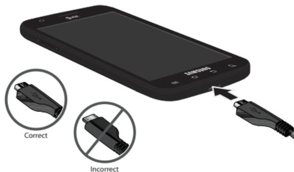
1. Plug the flat end of the Travel Charger into the Power/Accessory Interface connector and the other end into a standard AC wall outlet.
