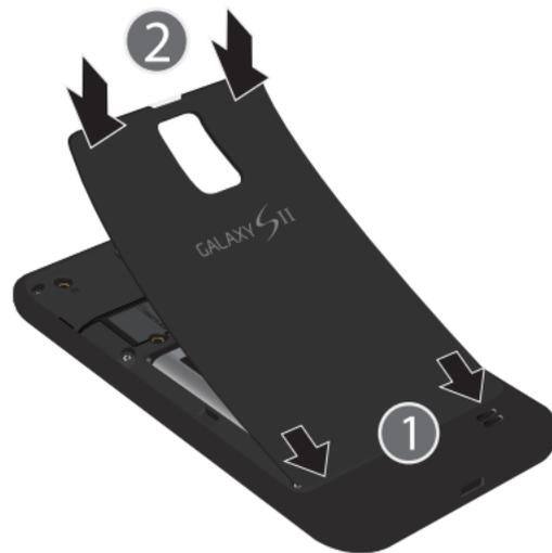
2. Press all along the edge of the back cover until you have a secure seal.
