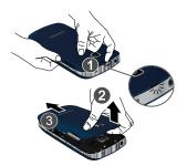
**3.** Lift the battery up (1) and away (2) from the phone, bottom end first.
