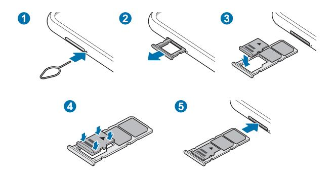
1 Insert the ejection pin into the hole next to the tray to loosen the tray.
