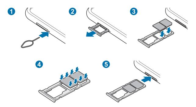
1 Insert the ejection pin into the hole next to the tray to loosen the tray.
