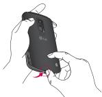
2 Then insert the micro SD card into the slot. Make sure the gold contact area is facing downwards.
