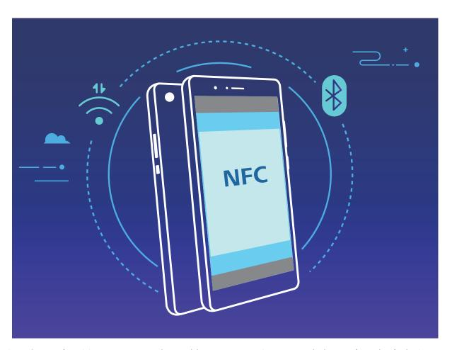
Using Bluetooth pairing as an example, enable NFC, Huawei Beam, and Bluetooth on both devices. Open the Bluetooth pairing screen on both devices and place the NFC detection areas of devices close together. When the sending device plays an audio prompt and content on the screen shrinks, follow the onscreen instructions and touch the screen on the sending device to establish a Bluetooth connection
