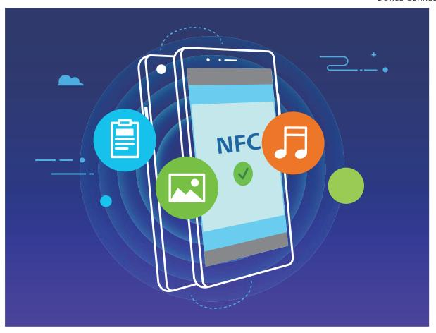
Use NFC to send data: Open Settings, touch Device connectivity and enable NFC and Huawei Beam. Select the files you want to send and touch Share > Huawei Beam. Keep your Phone unlocked and the screen on. Place the NFC detection areas of both devices close together. Once a connection is established, the transmitting device will play an audio alert and minimize the sharing screen. Touch the transmitting device's screen to send files.
