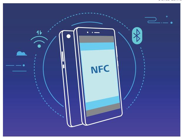
Using Bluetooth pairing as an example, enable NFC, Huawei Beam, and Bluetooth on both devices. Open the Bluetooth pairing screen on both devices and place the NFC detection areas of devices close together. When the sending device plays an audio prompt and content on the screen shrinks, follow the onscreen instructions and touch the screen on the sending device to establish a Bluetooth connection
