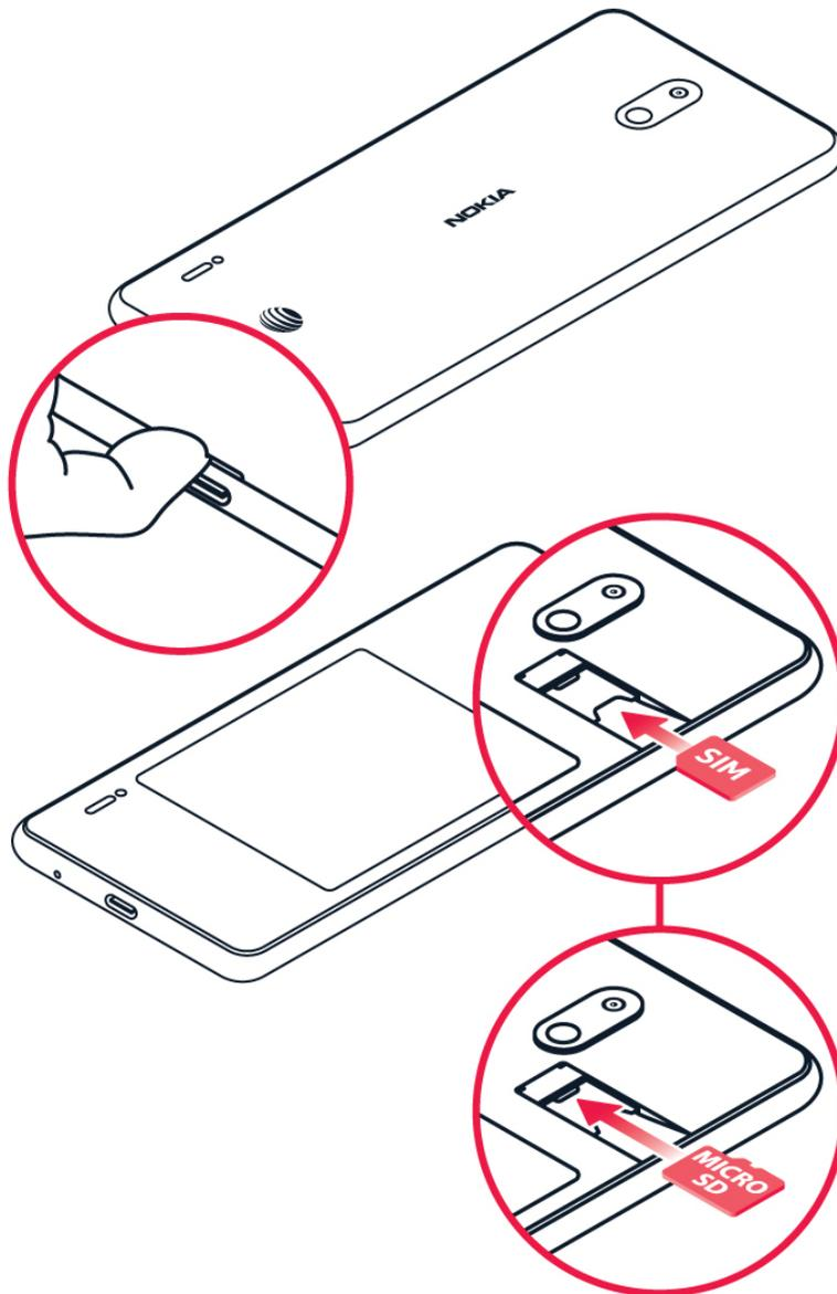
1. With the phone facing down, put your fingernail in the small slot on the back cover, bend the back cover open, and remove it.
