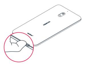
Slide the microSD card into the microSD card slot with the gold contacts facing down.
