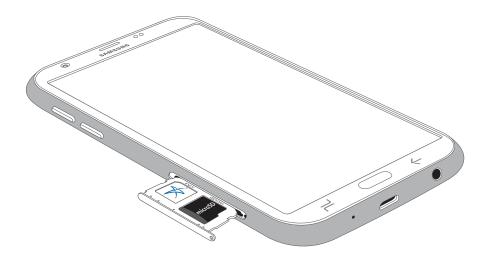
4. Slide the SIM card/Memory card tray back into the slot.
