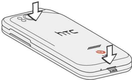
2. Press the sides of the back cover down to lock it into place. You'll hear clicks when the small tabs underneath the back cover are locked in place.
