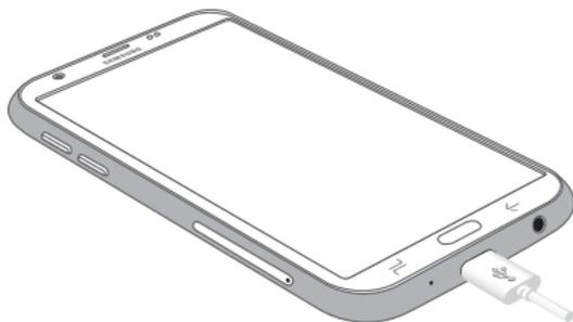
2. Connect the USB cable to the charging head, and then plug the charging head into a standard outlet.
