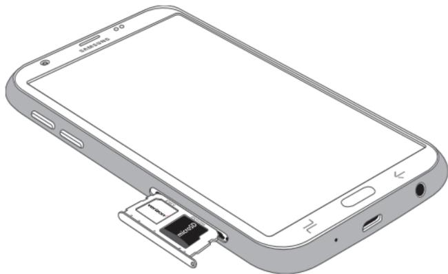
4. Slide the SIM card/Memory card tray back into the slot.
