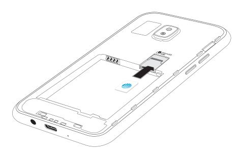
2. Slide the memory card into the slot with the gold contacts facing down.
