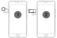
2. Insert the SIM card(s) and SD card, as shown:
