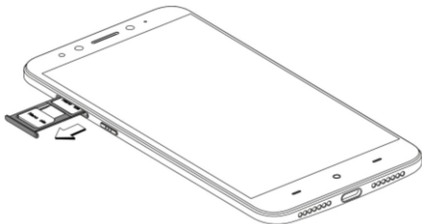
2. Insert the SIM card(s) and memory card into the tray as shown:
