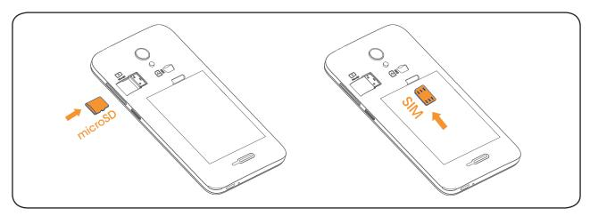
3. Ensure that SIM and microSD cards have been properly secured.
