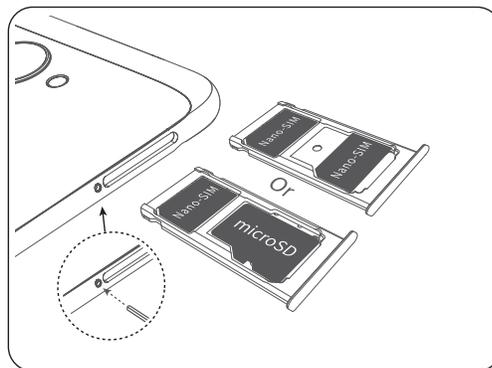
**3** Insert a SIM card or microSD card into the card tray.
