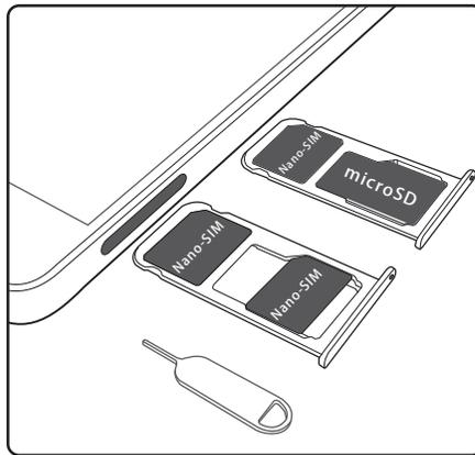
**3** Insert a SIM card or microSD card into the card tray.
