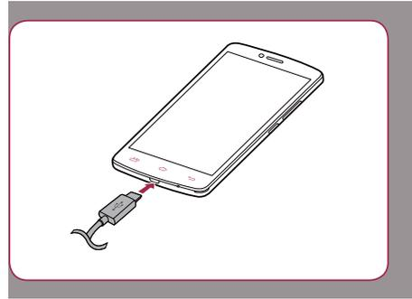
1. Plug the small end of the charger into the micro USB port of the device, and plug the large end of the charger into an electric socket.
