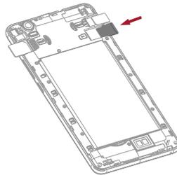
**5** Insert the battery into the battery compartment.
