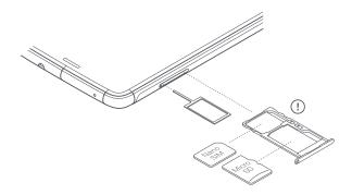
Insert the point of the SIM key into the ejector hole.
