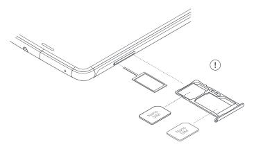
The SIM key is found in the device's box. Ensure the device is switched off, then extract the tray by inserting the key into the hole beside the SIM slot. Place the nano-SIM card on the tray. Ensure correct positioning by aligning the notch on the card with that on the tray (see image). Insert the tray and nano-SIM into the slot.
