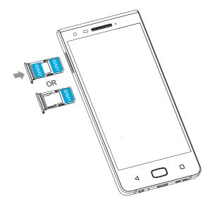
5. Push the SIM/microSD tray back into the slot.
