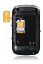
Slide the SIM card into the slot.
