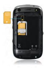
Slide the SIM card into the slot.
