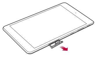
2 Put the Nano-SIM card and a microSD card (optional) on the card tray, then slide the card tray into the slot as shown in the figure below. Make sure the gold contact area on the card is facing downward.
