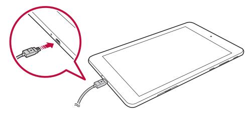
Charge the battery before using it for the first time. Use the charger included with your device to charge the battery. A computer can also be used to charge the battery by connecting the device to it using the USB cable.
