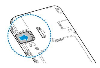
Hold the microSDXC card with the metal contacts facing down and the cut corner oriented a shown, and slide it into the card slot.
