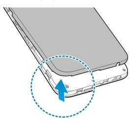
2. Hold the nano-SIM card with the cut corner oriented as shown and slide it into the card slot.
