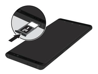
4. Slide the SIM card/Memory card tray back into the slot.
