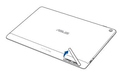
2. Press the memory card to eject, then pull it out.
