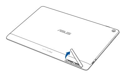
2. Press the micro SIM card to eject, then pull it out.
