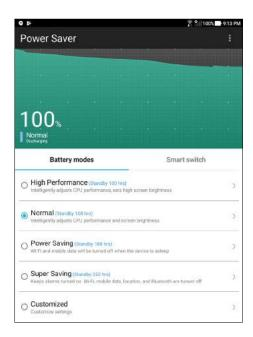
3. For advanced settings, tap **Smart switch**. Then you can choose **Switch according to battery level** or **Switch according to schedule** for more options.
