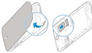
1. Place your finger in the slot at the bottom of the back cover to lift and remove the cover.
